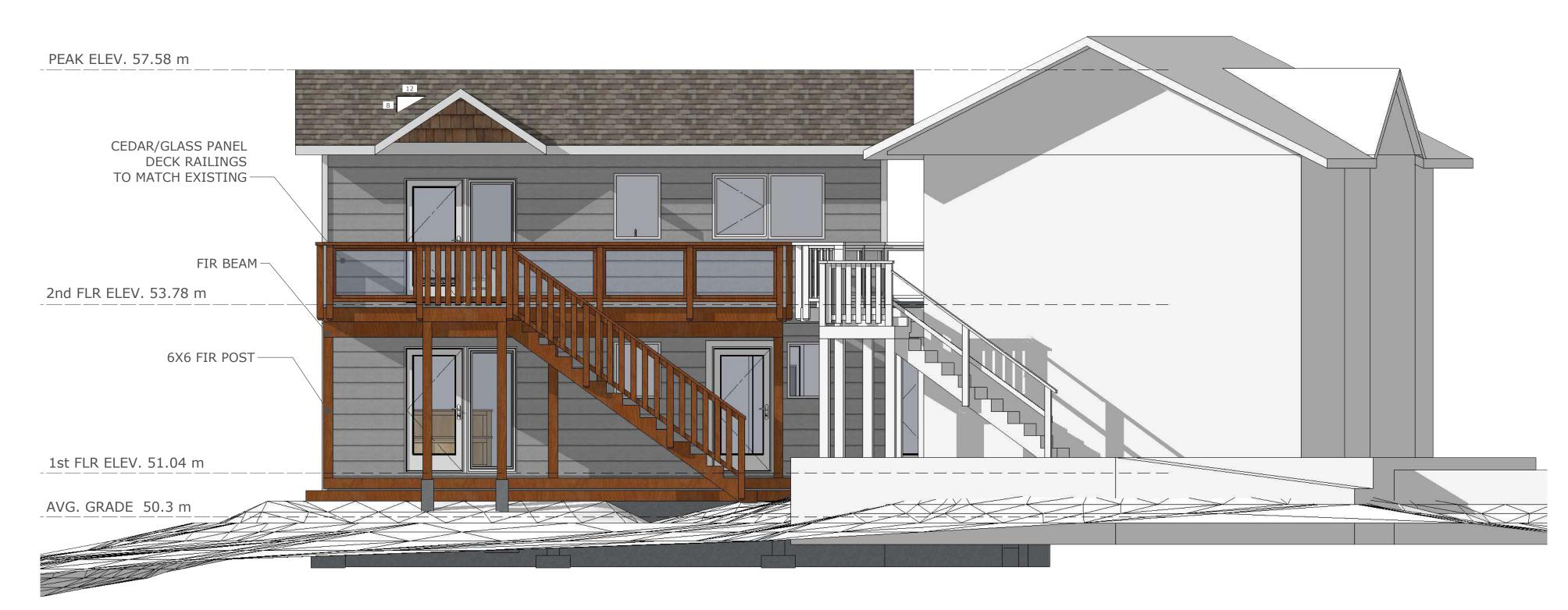
SOUTH ELEVATION (SIDE) - SCALE: 1/4" = 1'-0"
